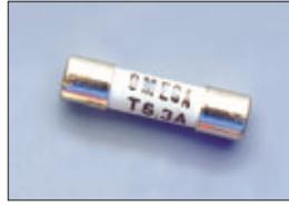
In compliance with IEC 60127-2-1 – rapid fusion – 250 V in steatite tube filled with arc-quenching powder (breaking capacity 1500 A).
