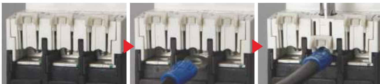
① Screw holder lifts up the screw
