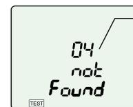
When incorrect wiring pattern cannot be detected
